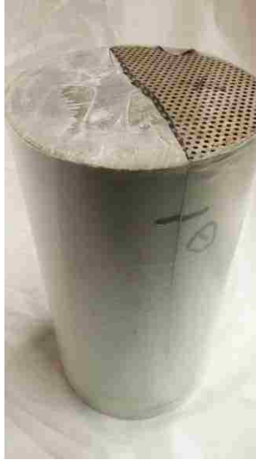
Figure 2.1. Fractured cement core with perforated sheets attached and wrapped with a release film
